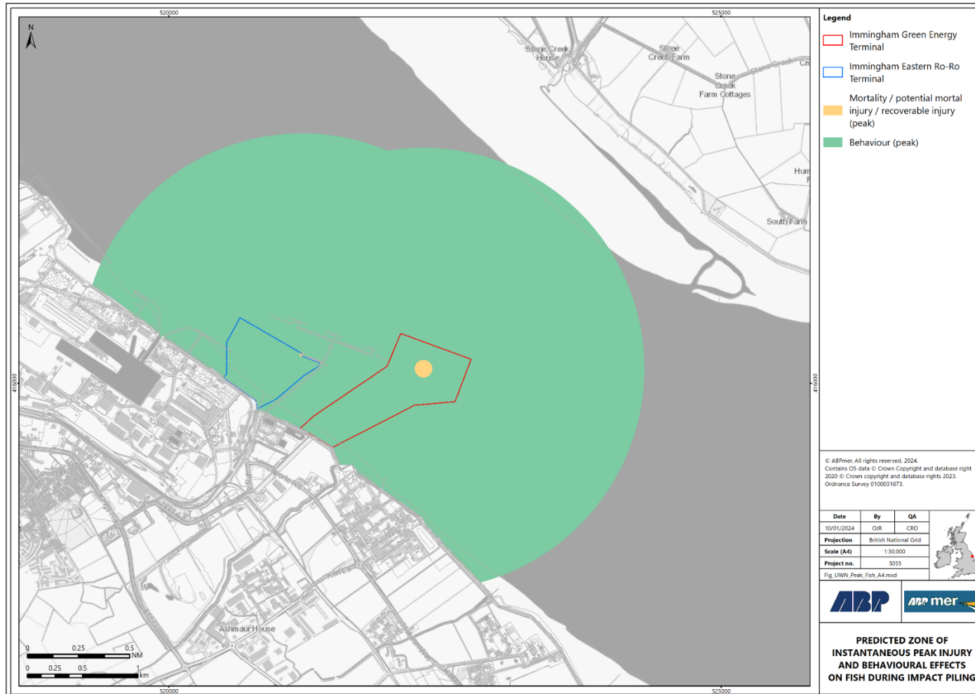
Figure 2. Predicted zone of instantaneous peak injury and behavioural effects on fish during impact piling
